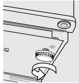
3. Compare the alignment of the appliance to the surrounding cupboard. The top of the appliance should be level from side to side (see diagram below). If you need to adjust the level, use the levelling feet as detailed in
