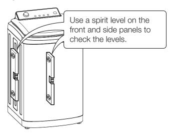
Tilt the washer a little to adjust the front legs.
