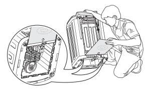
**3.** Lie down the washing machine on its back side, taking care not to damage cabinet by
