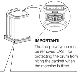
**NOTE:** After lifting the machine out, please check packaging base as below:
