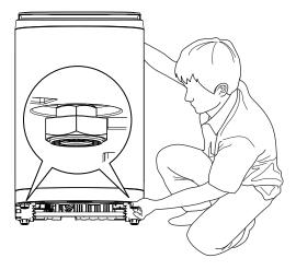
2. If you do not have a spirit level, as a guide use the edge of a door frame, cupboard or bench to check that the washing machine is levelled.
