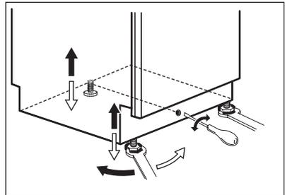
3. To adjust the rear height of the appliance, turn the middle screw counterclockwise.
