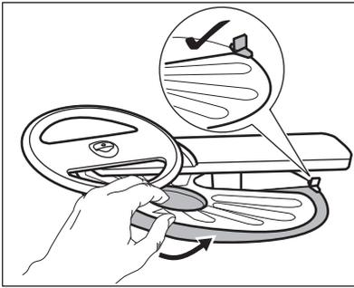
7. Reassemble the filters (B) and (C).
