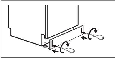
Once the installation is completed, make sure that the bottom of the adjustable plinth is aligned with the floor.
