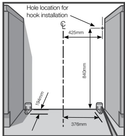
Measurements are to be adjusted to account for the thickness of any skirting board or tiles coming between the back of the appliance and the wall
