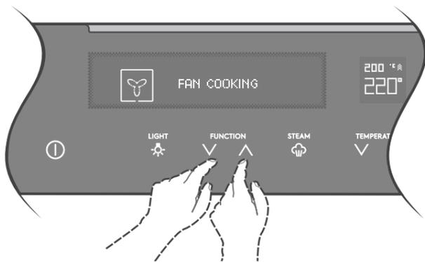
4. Activate the Steam button by touching . The steam control works only with the 'Fan cooking' function.
