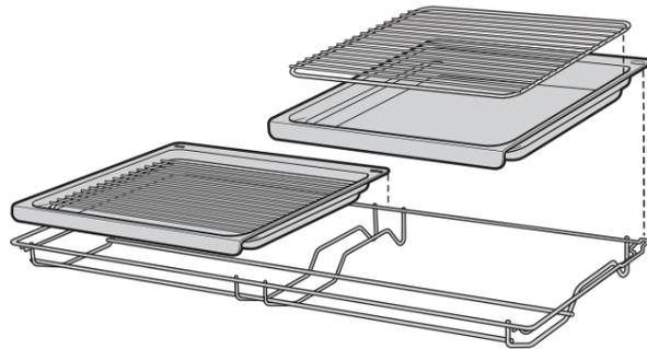
**Fitting the shelves and grill dish carrier onto telescopic slides**
