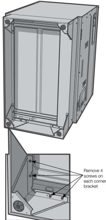
Remove 4 screws on each corner bracket
