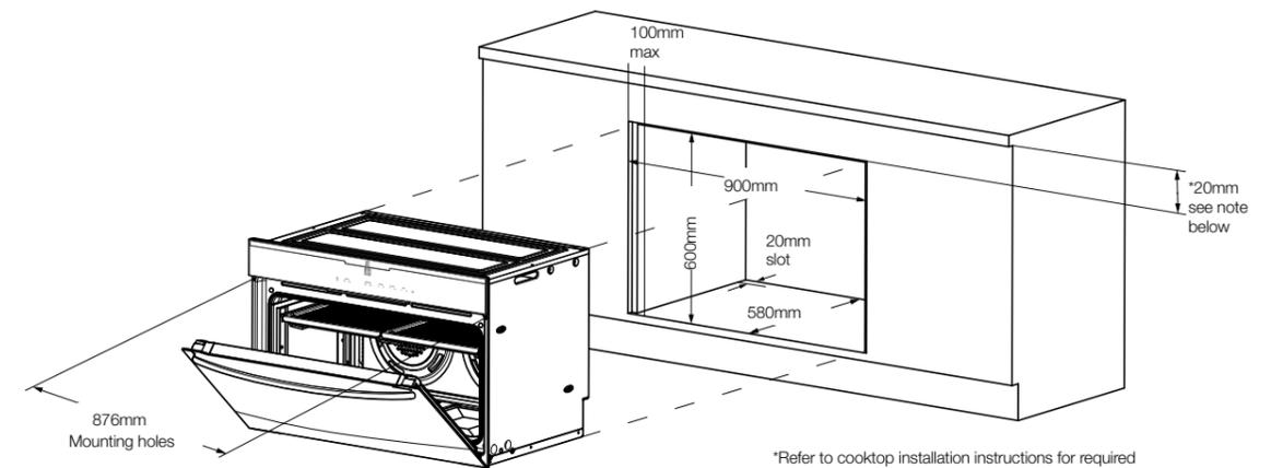
*NOTE: If a powerpoint is fitted it must be accessible with the appliance installed.*
