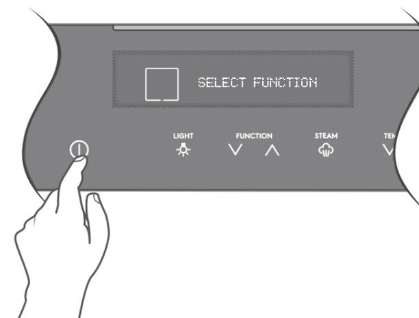
2. **Select a cooking function** by pressing the function or function as many times as necessary until the desired function appears.
