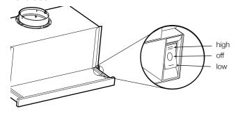
To switch on the rangehood light, use the switch located on the left hand side of the rangehood.
