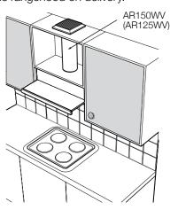
Carbon filters diminish cooking odours in the recirculated air. Depending on the frequency of use and the type of cooking, the expected life of carbon filters is 1-6 months. Using carbon filters with reduce the airflow of the rangehood.
