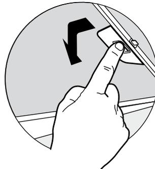
Switch off the electricity! Remove the plug from the socket or switch the electricity off at the mains. Open the panel and pull the special handle to remove the filter.
