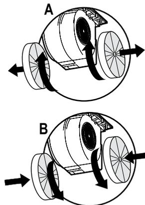
The carbon filter must always be used if the cooker hood is not ducted.
