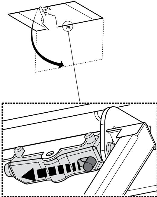
2. Remove the grease filter.
