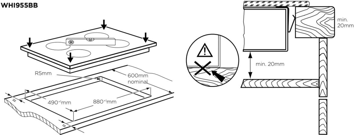
It is recommended to centre the bench cutout with equal distance front and back as shown but the product has also been certified to be installed with no clearance between the rear edge of the cooktop glass and rear wall if required. In doing so installers still need to leave sufficient clearance to take into account that the glass dimensions are larger than the cut out
