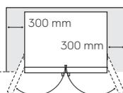
When positioned in a corner area, spacing of at least 300mm on the hinge side will allow the doors to open enough to enable the removal of bins and shelves.
