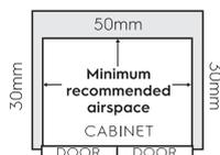
**Please note:** If 5mm side clearance, the fridge cabinet must sit at least 5mm proud of kitchen cabinetry for doors to open. A 5mm side clearance requires 50mm rear clearance and 50-90mm clearance above.
