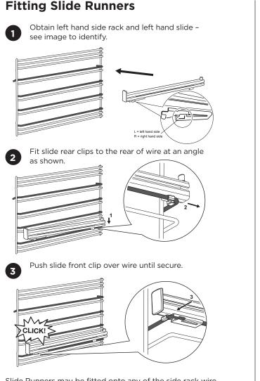
Slide Runners may be fitted onto any of the side rack wire positions as highlighted.
