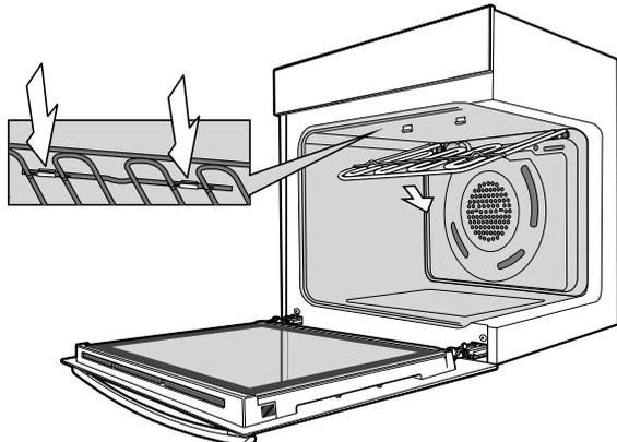
Rotating latch models - rotate latch 180° and the grill element will drop down freely. After cleaning, raise the grill element and secure by rotating the latch back 180°.
