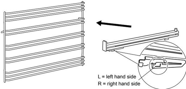
2. Fit slide rear clips to the rear of wire at an angle as shown below.
