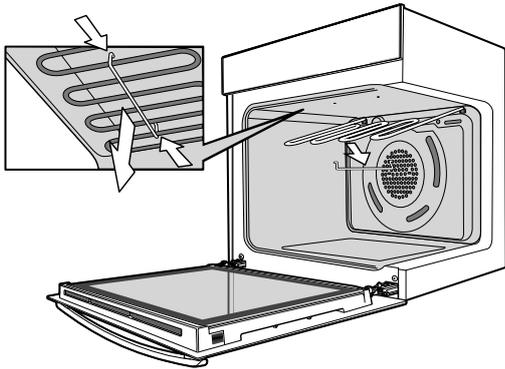
Retaining clips models - The upper grill element is secured with 2 clips which can be removed to help clean the oven cavity ceiling. To disengage the clips, push the edge of the clip towards back of the oven as shown below. After cleaning raise the grill element and secure clips back in position.
