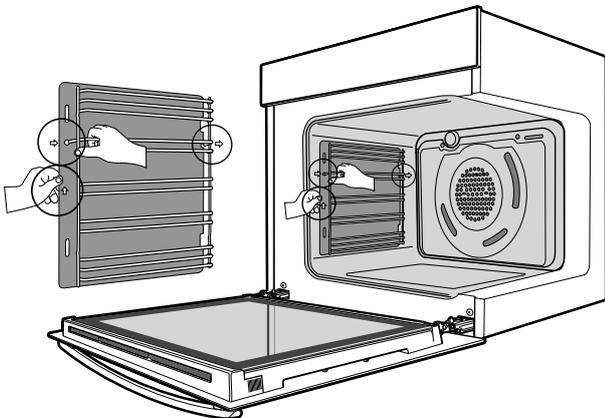
**Removing catalytic liners (where fitted)**
