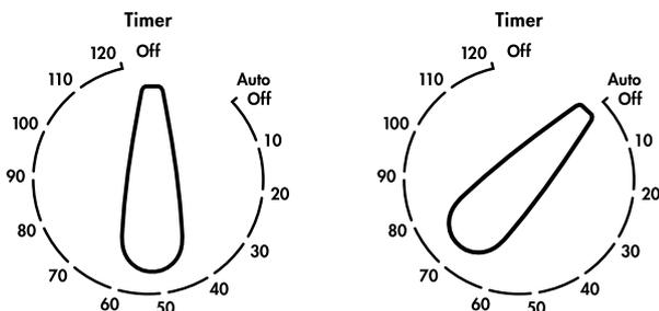
Once automatic baking is complete, return to manual operation by setting the timer to the “OFF” mark.
