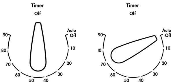
Once automatic baking is complete, return to manual operation by setting the timer to the “OFF” mark.
