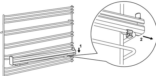
3. Push slide front clip over wire until secure.
