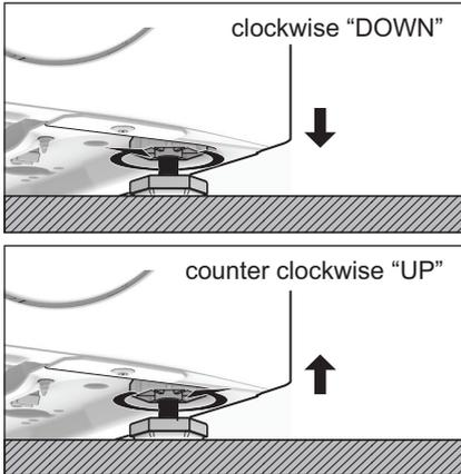
When the washing machine is levelled, try to rock it from corner to corner. If it does rock, adjust the legs again until it is levelled and does not rock.
