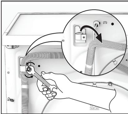
4. Put the end of the drain and inlet hose in a container. Let the water flow out of the hoses.
