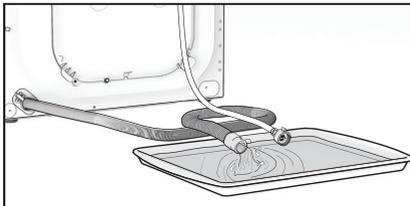
5. When no more water flows, install the inlet hose and the drain hose again.
