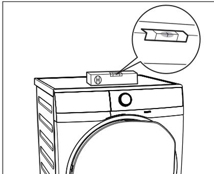
If you do not have a spirit level, as a guide use the edge of a door frame, cupboard or bench to check that the washing machine is leveled.
