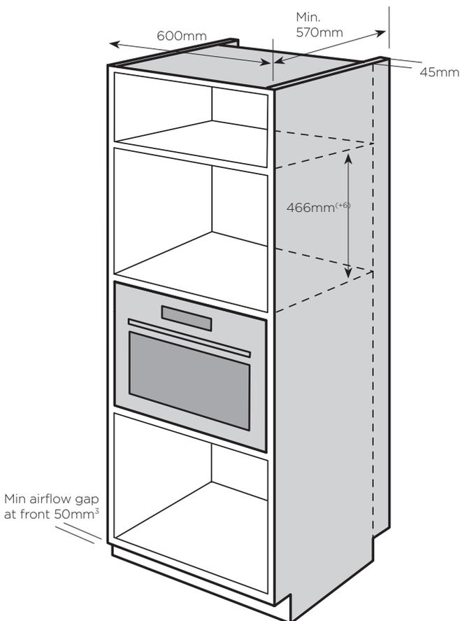
A 45mm ventilation gap must be left between the built-in cabinetry and wall with no back panelling on the cabinet housing the microwave oven. A minimum ventilation gap of 3.5mm must be left between the bottom of the front trim and adjacent shelf/cupboard.
