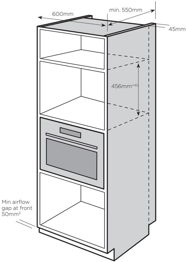
A 45mm ventilation gap must be left between the built-in cabinetry and wall with no back panelling on the cabinet housing the microwave oven.
