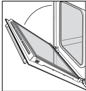
3. Grasp the oven door with a hand each side of the door and remove it from the oven by pulling it towards you.
