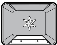
Heat comes from the gas “base heat” burner which is then circulated by the fan. This fan circulates the hot air around the oven cavity so that you can put your food in different places in the oven and still cook them at the same time.
