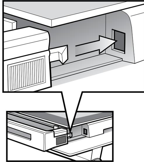
3. Push the middle of the trim down to ensure it is straight and firm against the glass panel.
