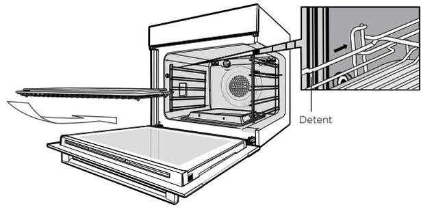
4. When fully inserted the shelf should not interfere with the closed oven door.
