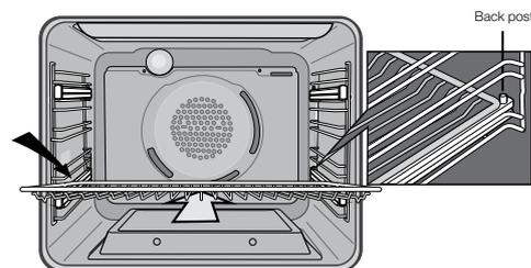
2. Drop the front of the shelf or tray onto the slide ensuring it sits behind the front post of the slide.
