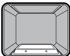
Heat comes from the gas “base heat” burner below the food. The bottom burner is below the floor of the oven which is controlled by the thermostat and will turn on and off to maintain the set temperature.
