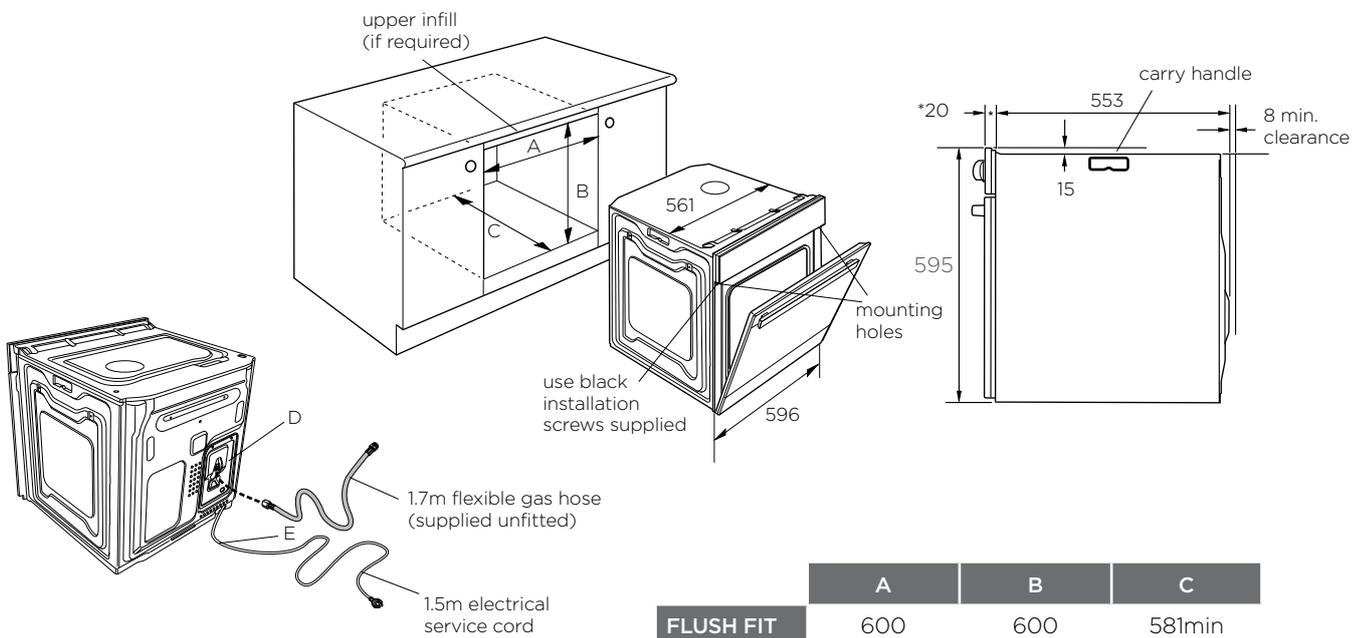
D Gas connection - 150mm from right hand side
