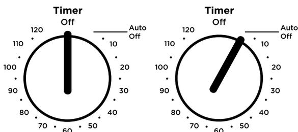
Once automatic baking is complete, return to manual operation by setting the timer to the "OFF" mark.
