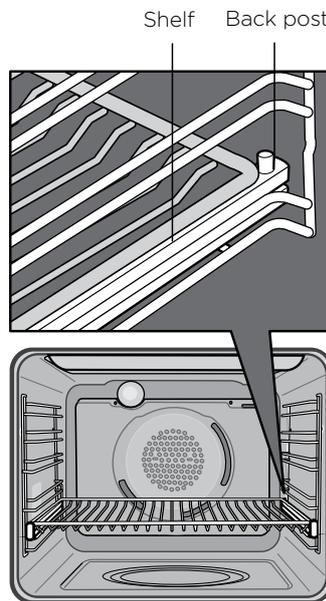
2. Drop the front of the shelf or tray onto the slide ensuring it sits behind the front post of the slide.
