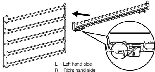
2. The shaded wires indicate the wire the slide can be mounted on. Fit slide rear clips to the rear of wire at an angle as shown below.
