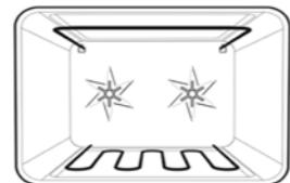
Heat comes from two elements, one above and one below the food. The fans circulate the hot air around the oven cavity so that you can put the food in different places in the oven and still cook them at the same time. You should only use a maximum of 2 shelves with "Fan Assist". Do not use the bottom shelf. If two shelves are used, food on the shelf in the higher position will cook first and should then be removed to allow the food on the lower shelf to finish cooking.
