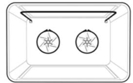
This function can be either used for a quicker pre-heat of your oven or used to turn your oven into an AirFry for your frying needs. Heat comes from the elements surrounding the fans as well as the smaller element above the food. This will heat up your oven 30% faster.
