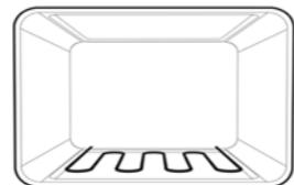
Heat comes from the element below the floor of the oven. The Element is controlled by the thermostat and will turn on and off to maintain the set temperature. The "Base Heat" function can be used to add extra browning to the bases of pizzas, pies and pastries. Cook in the lower half of the oven when you are using only one shelf. For best results, use silver or shiny trays.
