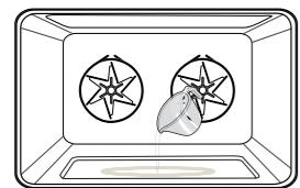
Easy Bake Steam adds humidity at the beginning of the baking process. In bakery products, this allows the dough to rise and helps create a moist interior while obtaining a golden and crispy crust. Before preheating, when the oven is cold, add water to the cavity well. Refer to chapter 'Easy Bake Steam' for more details. For best results preheat the empty oven for 10 minutes prior to inserting food.
