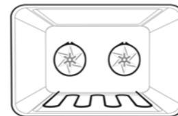
"Pizza" is a combination of "Base Heat" and "Fan Forced" and offers you the combined benefits of both functions. Heat comes from the elements surrounding the fans as well as the clean heat element below the oven floor.
