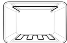
Heat comes from two elements, one above and one below the food. The bottom element is a clean heat element and is below the floor of the oven. Both elements are controlled by the thermostat and will turn on and off to maintain the set temperature. You can use the "Bake/Pizza" function for pizza and single trays of biscuits, scones, muffins, cakes, slices, casseroles, baked puddings, roasts and delicate egg dishes.
