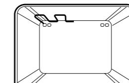
The 'Left Grill' directs radiant heat from only one of the powerful upper elements onto the food. The 'Left Grill' function is used instead of 'Full Grill' when only half the amount of grill area is needed. Left Grill has 2 temperature settings, 'LO' and 'HI'. Grill with the oven door closed.'
