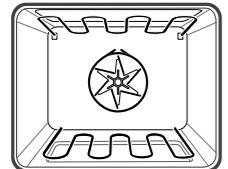
The Roast Function is designed for roasting meats and poultry by utilising heat from all elements in combination with the fan to surround the food. This provides even cooking throughout and enhanced browning. This function starts at a higher temperature to seal the meat. The oven will then automatically reduce to the selected temperature to cook the meat for as long as desired. For example, if you use the default 200°C the "Roast" cycle will start at 220°C and then lower to 200°C.
