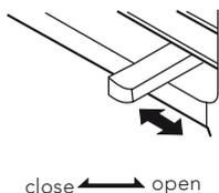
To open the vent, push the lever to the right.
