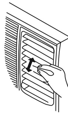
To adjust vertical air flow direction, adjust any one of the horizontal louvre blades. When turning the horizontal louvre blades up or down, always keep the top or bottom blades horizontal. This can effectively prevent water drops condensed on the front panel of the unit.
