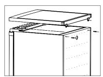
2. Remove the four screws as shown in the diagram. Remove the top hinge and keep for reassembly.
