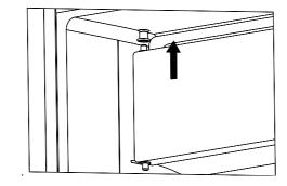
5. Keep the freezer compartment door closed. Fix the installation button to the lower door bearing, Press the installation button to make it have no gap with the cavity, then fix the screw.
