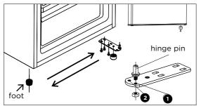
4. Set the door into its new place making sure the pin enters the bushing at the lower frame section. Replace the lid by fitting the upper hinge into the upper door's hole, securing it with the two screws. Replace another two screws to another side.
