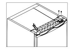
5. Replace the top cover. Tighten the two screws on the back of top cover.
