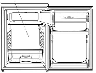
Turn the control knob clockwise to turn the appliance on. Rotating clockwise will make the appliance colder.
