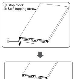
Lay the refrigerator on soft foam packaging or similar material. Remove both adjustable bottom feet parts, and the lower hinge part by unscrewing the special flange selftapping screws.
