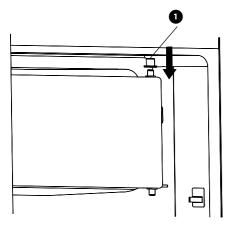
3. Using a screwdriver, take down the installation buckle, and then fix it in the opposite side.
