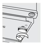
3. Compare the alignment of the appliance to the surrounding cupboard. The top of the appliance should be level from side to side (see diagram below). If you need to adjust the level, use the levelling feet as detailed in step 2.
