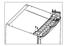
Lift the door and place it on a padded surface to prevent scratching. Remove both adjustable feet and remove the bottom hinge bracket by unscrewing the bolts. Then transfer them to the other side.
