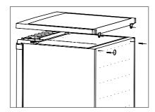
replace note copy to read: "Note: 1. You need to move the hinge pin from hole 1 to 2 before transfer. 2. You need to install the foot on the side which does not have a hinge."
