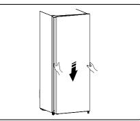
9. Transfer the upper hinge part and make the upper hinge axis into the upper hole of the door, and adjust the position of the door(please support the door with your hand when doing it), fixing the upper hinge part with the special flange self-tapping screws.
