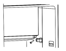
Open the freezer compartment door a little way. Pull down the freezer compartment door and the cap which covering on the up door bearing 1.
