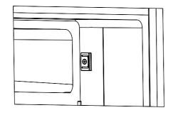
4. Turn the freezer compartment door through 180°, cover the cap on the up door bearing, then fit the door into the up door axle hole.
