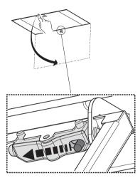
2. Remove the grease filter.
