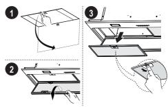
Switch off the electricity! Remove the plug from the socket or switch the electricity off at the mains. Open the panel and pull the special handle to remove the filter.
