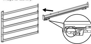
The shaded wires indicate the wire the slide can be mounted on. Fit slide rear clips to the rear of wire at an angle as shown below.
