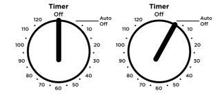
Once automatic baking is complete, return to manual operation by setting the timer to the "OFF" mark.
