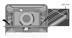
2. Drop the front of the shelf or tray onto the slide ensuring it sits behind the front post of the slide.
