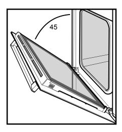
Grasp the oven door with a hand each side of the door and remove it from the oven by pulling it towards you.
