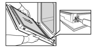
Lay the oven door with the outer side facing downwards on something soft and flat (for example a blanket on a kitchen table) to prevent scratches.
