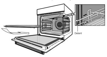
4. When fully inserted the shelf should not interfere with the closed oven door.
