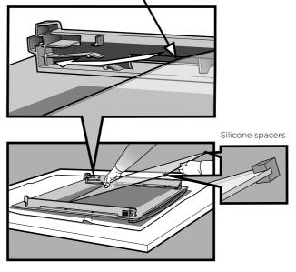
Insert the remaining smaller clear glass panel into the middle position, ensuring the chamfered corner of the panel is placed in the correct location as shown in the image below.
