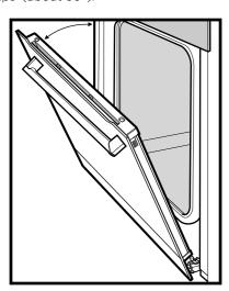
Hold the oven door with a hand each side and remove it from the oven by pulling it towards you.
