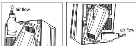
Inlet and outlet points need clear airflow to prevent overheating, so ensure there is adequate ventilation. (i.e. open window or external door.)
