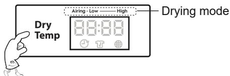
Touch this touch pad to select the drying mode. Corresponding light for each mode is shown on display. Drying mode can only be selected during initial set up.
