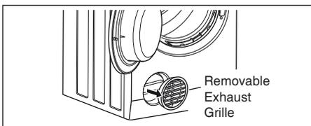
**Do not install your dryer in a cupboard or small un-vented laundry unless you are using a venting kit.**
