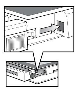
• Push the middle of the trim down to ensure it is straight and firm against the glass panel.
