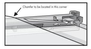
• Insert the black bordered glass panel into the upper position, ensuring the painted surface is facing the downside as per the diagram below..
