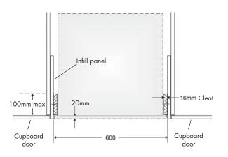
Figure A - Flush fit (top view)
