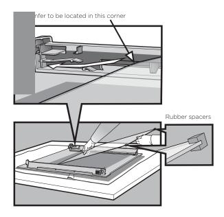
• Insert the remaining smaller clear glass panel into the middle position, ensuring the chamfered corner of the panel is placed in the correct location as shown in the diagram below.
