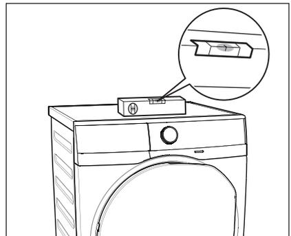
If you do not have a spirit level, as a guide use the edge of a door frame, cupboard or bench to check that the machine is leveled.
