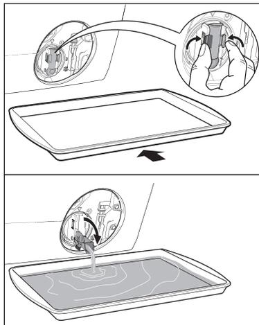
3. When the container is full of water, put the drainage duct back again and empty the container. Do step 2, 3 again and again until no more water flows out from the drain pump.
