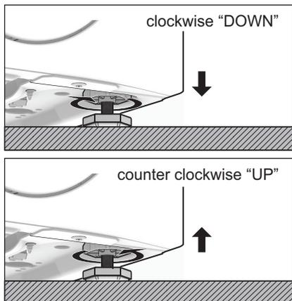
When the Washer-Dryer is levelled, try to rock it from corner to corner. If it does rock, adjust the legs again until it is levelled and does not rock.
