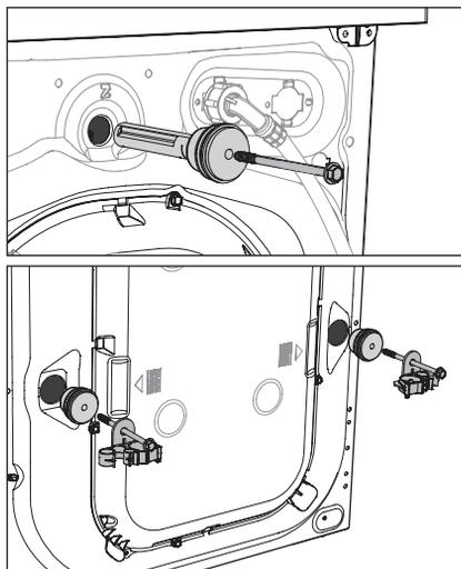
**!** Transit bolts must be removed before using the appliance.
