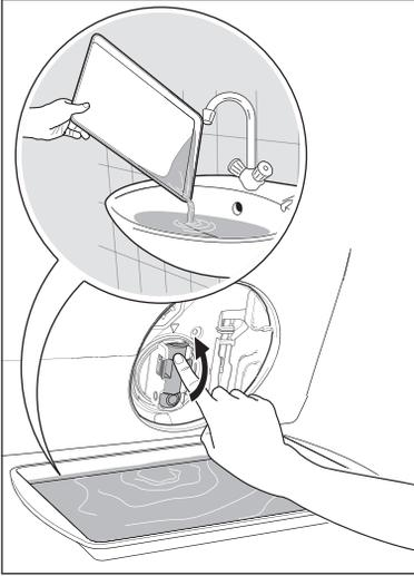
4. Push back the drainage duct and turn the filter counter-clockwise to remove it.
