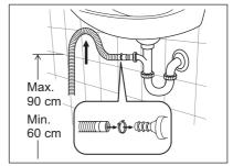
Push the drain hose onto the spigot and secure with a clamp, ensure a loop is formed in the drain hose to prevent waste from the sink entering the appliance.
