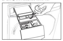
3. Gently pour only liquid detergent in the AutoDose detergent tank 🔊. Fill up to the maximum indicated level MAX.
