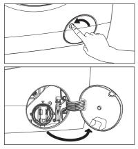
Place a suitable water container below the recess of the drain pump to collect the water that flows out.
