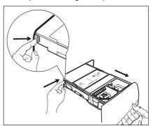
Remove the insert for the softener and, if inserted, the special container for liquid detergent.
