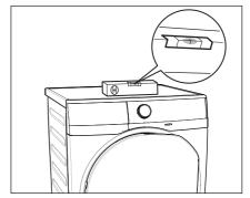
If you do not have a spirit level, as a guide use the edge of a door frame, cupboard or bench to check that the machine is leveled.
