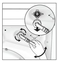
5. Use a suitable tool pulling filter from the valve (eg. long nose pliers) as picture.
