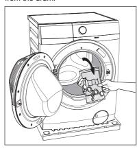
Put one of the polystyrene packaging elements on the floor behind the appliance. Carefully put down the appliance with the rear side on it. Make sure not to damage the hoses.
