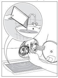
Push back the drainage duct and turn the filter counter-clockwise to remove it.
