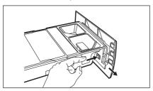
Make sure that all detergent residue is removed from the upper and lower part of the recess. Use a small brush to clean the recess.
