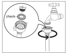
The inlet hose must not be lengthened. If it is too short and you do not wish to move the tap, you will have to purchase a new, longer hose specially designed for this type of use.
