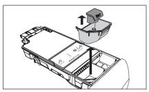
3. Open the drain plugs of each tank and empty them into a sink.
