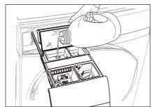
4. Gently pour only liquid softener in the AutoDose fabric softener tank 89. Fill up to the maximum indicated level MAX.
