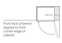
When positioned in a corner area, spacing of at least 350mm on the hinge side will allow the doors to open enough to enable the removal of bins and shelves.
