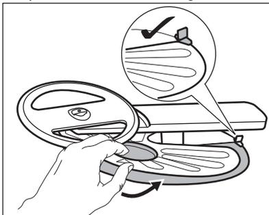
7. Reassemble the filters (B) and (C).
