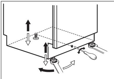
2. To adjust the rear height, turn the middle screw counterclockwise to raise the appliance.
