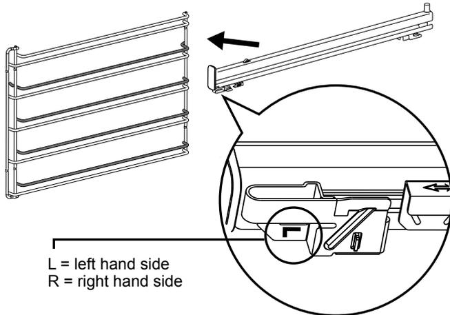
The shaded wires indicate the wire the slide can be mounted on. Fit slide rear clips to the rear of wire at an angle as shown below.
