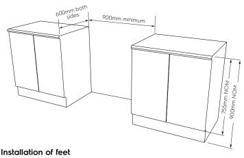
Freestanding appliances are supplied with four screw-in feet in the internal accessory pack. The screw-in feet can be adjusted by turning the lower half clockwise or anti-clockwise.
