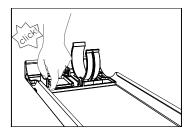
Make sure both clip modules are in the same orientation after installation.
