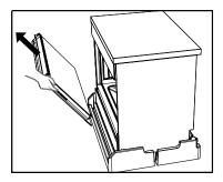
3. Tilt and carefully lay the appliance on its back to gain access to the installation point for the screw in feet.
