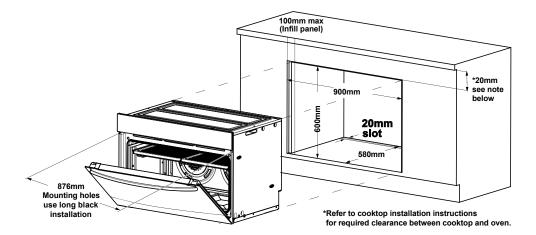
NOTE: If a powerpoint is fitted it must be accessible with the appliance installed.
