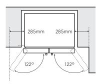
When positioned in a corner area, spacing of at least 285mm on the hinge side will allow the doors to open enough to enable the removal of bins and shelves.
