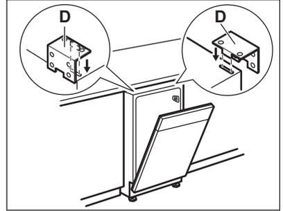
2. Install the appliance under the counter. Make sure that the appliance is levelled properly.
