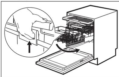
Once the basket is unlocked, push the rack down. The mechanism returns to its default position on the lower level.
