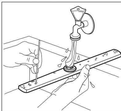
4. To install the spray arm back, press the spray arm upwards and simultaneously turn it counterclockwise until it locks into place.
