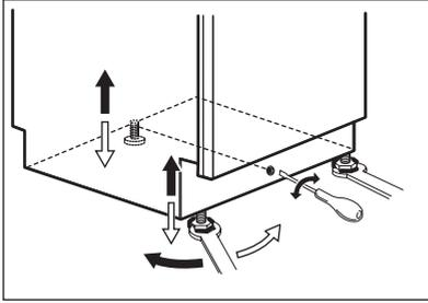
3. To adjust the rear height, turn the middle screw counterclockwise to raise the appliance.
