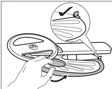
7. Reassemble the filters (B) and (C).
