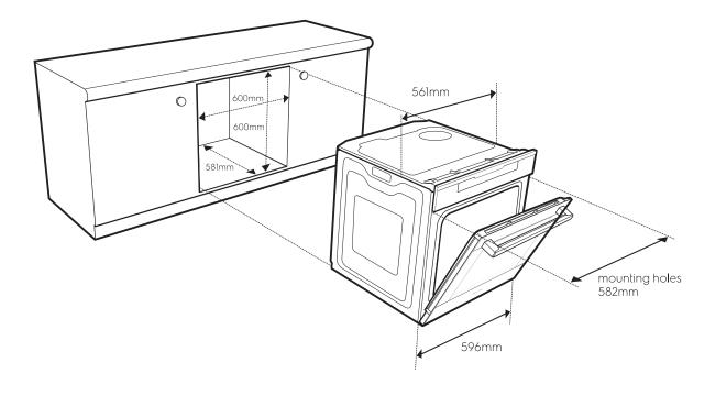
Please note! Dimensions to be used as a guide only. All customers MUST refer to the user manual supplied with the product for detailed installation instructions. © 2021 Electrolux S.E.A PTE. LTD. E\_DIM\_EVEP618DSE\_Sep21
