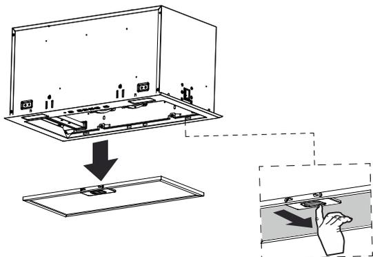
2. Unscrew the face panel screws from body and release the terminals of button and lights
