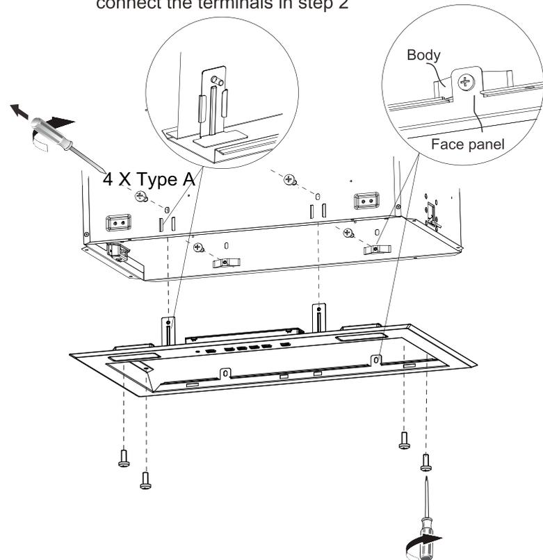
NOTE: Customer can adjust 4 screws (type A) to reduce the gap between hood body and cabinet
