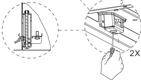
4. Fix the range hood using the supplied screws to fix the range hood.
