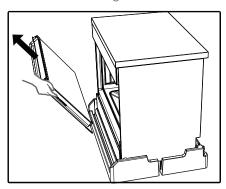
Tilt and carefully lay the appliance on its back to gain access to the installation point for the screw in feet.
