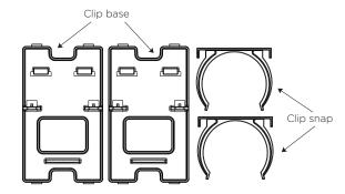
Assemble the clip snap onto the base.
