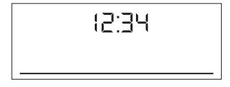
When the knob for the heating functions is in the off position, the display goes to standby.
