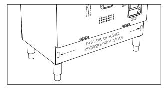
The following steps must be followed to ensure the correct installation of anti-tilt brackets and the stability of the appliances.
