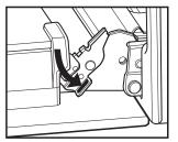
Locking tab up - normal position Locking tab down - for cleaning
