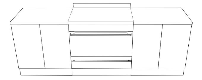
The slot-in type installation use the appliance as supplied. The appliance can be mounted on a plinth. This enables a continuous cupboard kickboard to be installed, giving a more integrated appearance. There is no clearance requirement between oven and adjacent side cabinets.
