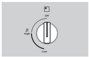
To light a burner with this knob, firstly depress and turn anti-clockwise to the 'High' flame position. The knob maybe released once the flame is established and turned further anti-clockwise to reduce the flame height as desired.
