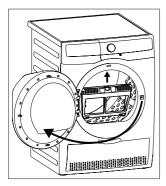
3. Insert the drying rack adapter.
