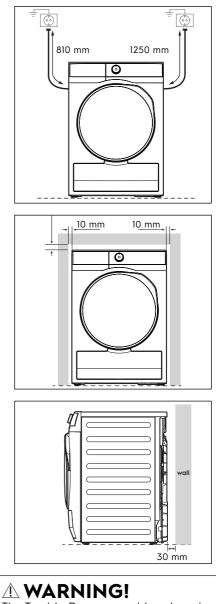
The Tumble Dryer cannot be placed directly on top of a washing machine without the use of an approved stacking kit. For more information, please contact authorised dealer.
