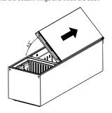
17. Replace LH centre hinge (kit content) by lifting the door slightly and sliding hinge into the door and placing the door down again.
