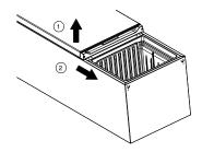
10. Remove bottom door by opening 45° and gently slide off hinge. Set door aside to prevent damage.
