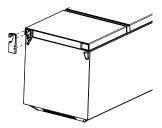
5. Remove the LH cap with a soft plastic lever.
