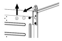
14. Place the bottom hinge LH (kit content) onto the cabinet, placing it down then towards cabinet to install. Replace the screw.
