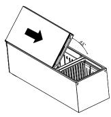
11. Remove the cover door from top door and assemble it on the other side. Remove the RH door auto closer and replace with LH door auto closer (kit content) on the other side. Repeat the same step with bottom door.
