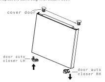
12. Unscrew the hinge foot using phillips head screwdriver and unscrew foot on opposite side. Do not discard.
