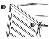
13. Unscrew the bottom hinge screw shown, pull the hinge away from cabinet then up to remove.
