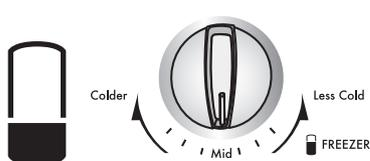
For top mount and bottom mount models, the coldest freezer setting is not recommended in normal or very hot climates. It will limit the cooling to the refrigerator section.
