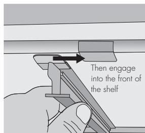
5. Fit the carriage by sliding it into the runners until the front of the carriage engages with the shelf.
