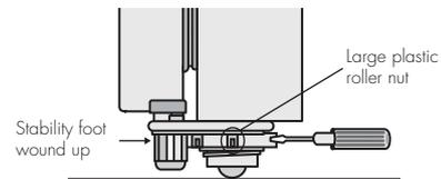
4. Check the alignment of the refrigerator to the surrounding cupboards to see if it is level. You can adjust the level with the rollers as detailed in step 3.
