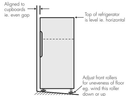
5. If you find your refrigerator rocks from corner to corner, it means your floor is uneven. Find a piece of plastic or hardboard etc. and pack it firmly under the roller.
