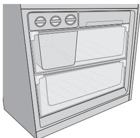
Freezer drawers are fitted to bottom mount models and single door all freezer models. The drawers are mounted on telescopic extension slides, to enable full access to the content in the drawer. Clear plastic fronts provide easy visibility of foods.
