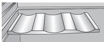
The bottle holder can be used to store various types of bottles like wine or beer. Bottles should be stored with the bottom end towards the back of the refrigerator. Electronic models are supplied with a chrome, full-width wine rack.
